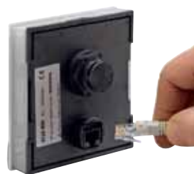
RJ45 to connect to ATyS p M
